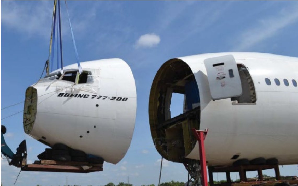
Figure 10 - 777-200 Line Number 30 Forward Section Removal (Images: Boeing)
